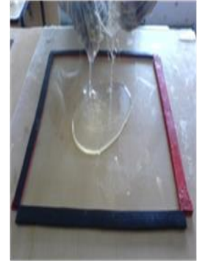
Applying resin to mold
